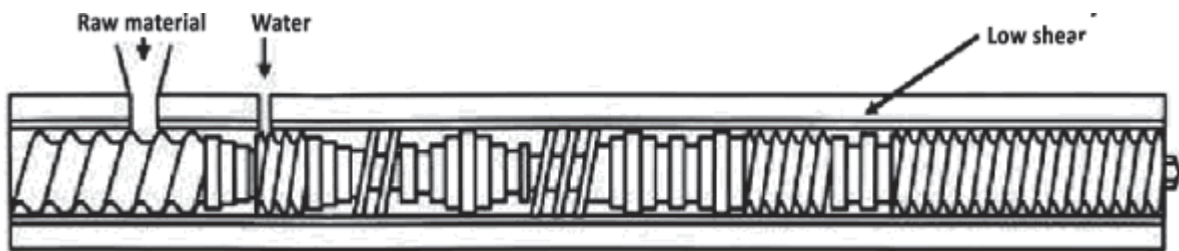
Fig. 1. Schematic representation of low shear screw configuration (Onwulata et al., 2001)
