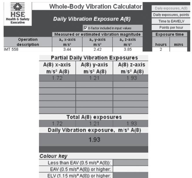
Fig. 2. HSE whole body vibration calculator-daily vibration exposure
