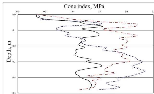
Fig. 5. The results of soil cone penetrometer resistance (cone index) in three measurement points (acquired using a sampling frequency of 2 Hz and an operating speed of  $10 \text{ mm s}^{-1}$ ) on the soil compacted after 20 tractor passes
