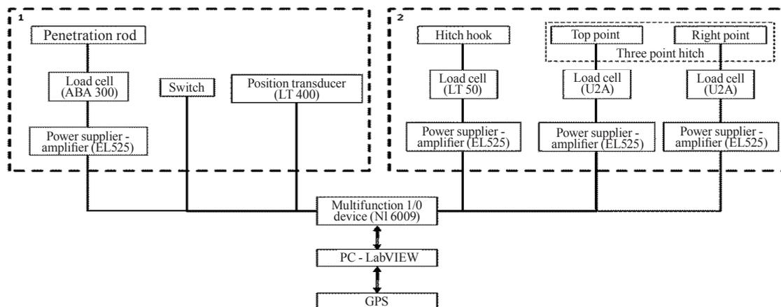
**Fig. 3. The scheme of the system for data acquisition: 1) system for acquiring the soil cone penetrometer resistance; 2) system for acquiring the draft force required to till the soil**
