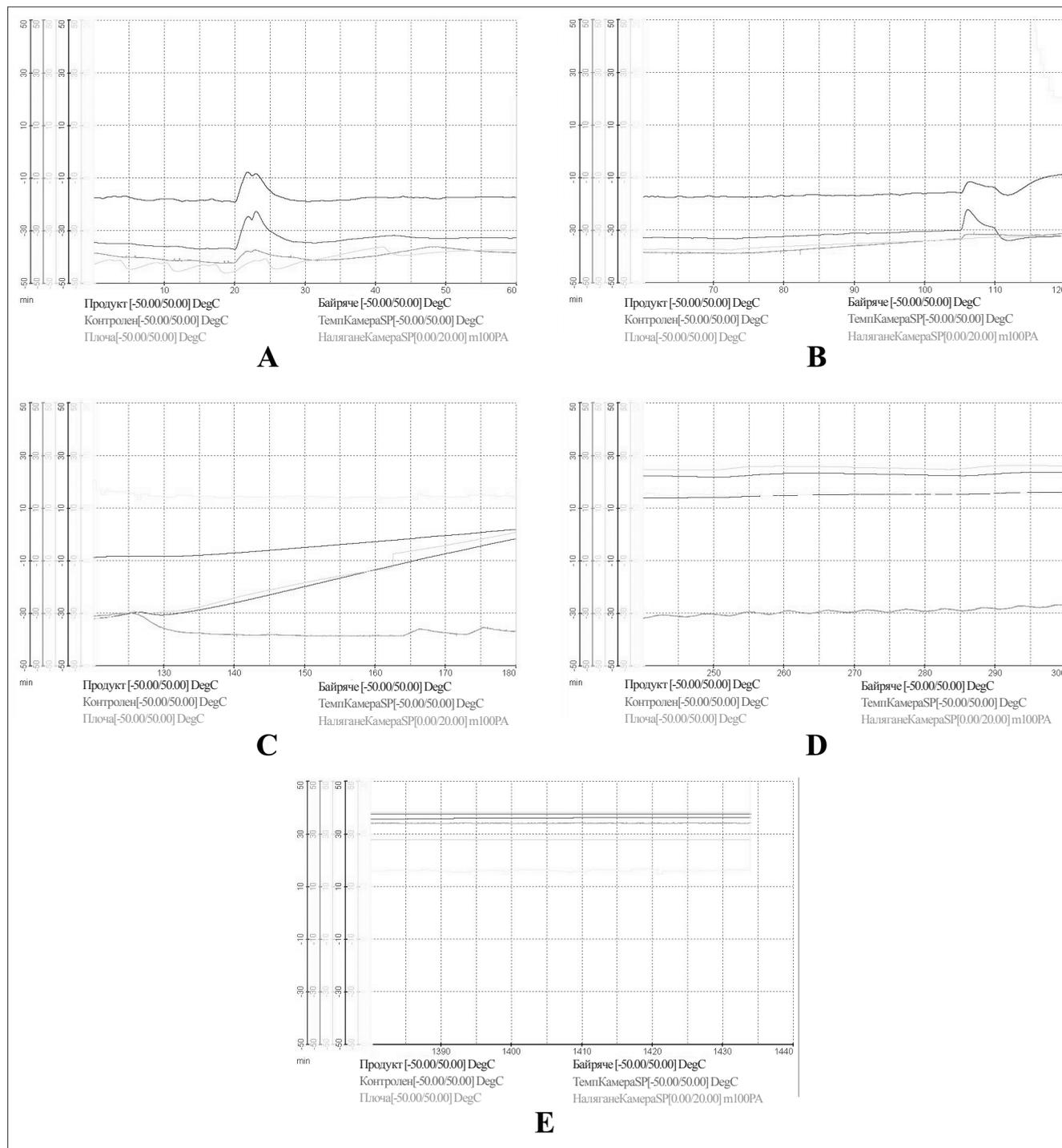
**Fig. 1. Record from the automatic controls during the process of lyophilization A-beginning of the process –freezing in a freeze-drying chamber; B- vacuum processing to deep vacuum  $2.10^1$  Pa; C – freeze-drying at negative temperatures; D – secondary drying – desorption of the residual moisture at positive temperatures and higher vacuum; E – end of the process – breaking of the vacuum, reaching of the limit final residual moisture**
