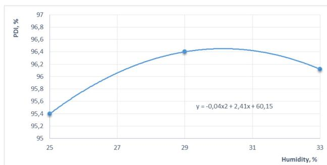
**Fig. 5. Effect of humidity of organomineral fertilizer on the strength of the granules obtained**
