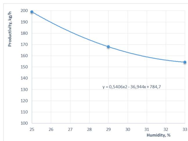
**Fig. 3. Effect of humidity of organomineral fertilizer on the performance of a pelletizing machine**
