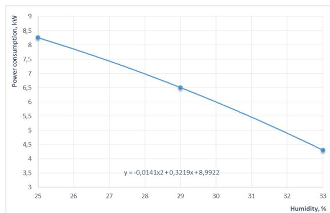
**Fig. 2. Effect of humidity of the organomineral fertilizer on power consumption**
