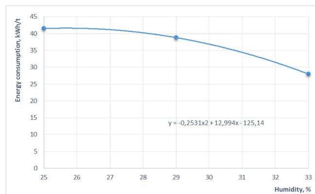
**Fig. 4. Effect of humidity of the organomineral fertilizer on the specific energy consumption of the pelletizing machine**
