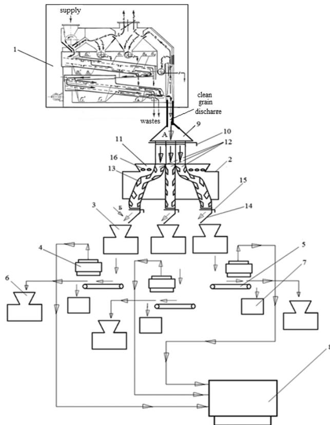
Fig. 1. Air-sieve grain-cleaning machine design
