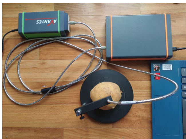
Fig. 1. The experimental setup used for the fluorescence spectroscopy. Measurements
